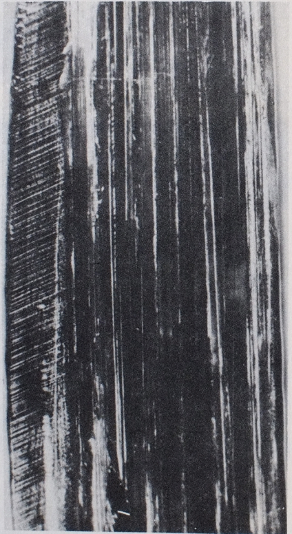
Phot. 6. Ridges formed at the flat ribbon surface at high growth rates
