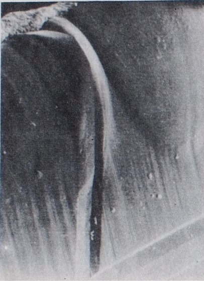
Phot. 5. Disturbance of the regular shape of ribbon observed at its lateral surface, due to the presence of a transverse twin boundary in the ribbon. SEM, \times 100
